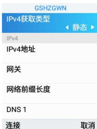
The screenshot shows a configuration menu for a device named 'GSHZGWN'. The 'IPv4获取类型' (IPv4 Acquisition Type) is set to '静态' (Static). Below this, there are input fields for 'IPv4地址' (IPv4 Address), '网关' (Gateway), '网络前缀长度' (Network Prefix Length), and 'DNS 1'. At the bottom, there are two buttons: '连接' (Connect) and '取消' (Cancel).
