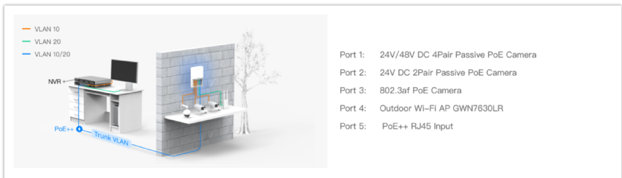
RJ45 Power and Data
