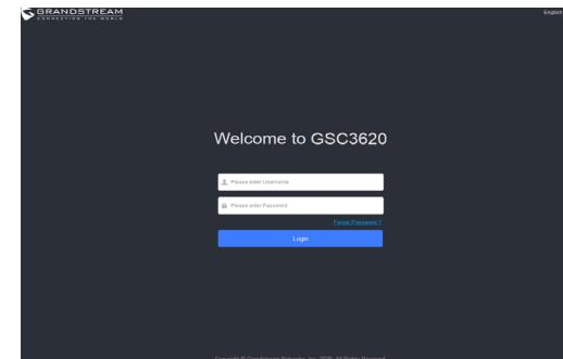
6. Username and password are required to login the camera to manage the device. The default username is "admin"; the default password is a random password printed in a sticker which can be found in the camera body and back of the QIG.
